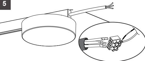
Thread the wires onto the ceiling and connect the corresponding wires using terminals.
